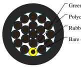
Green/Yellow wire Polychloroprene rubber outer jacket Rubber insulation Bare copper conductor
